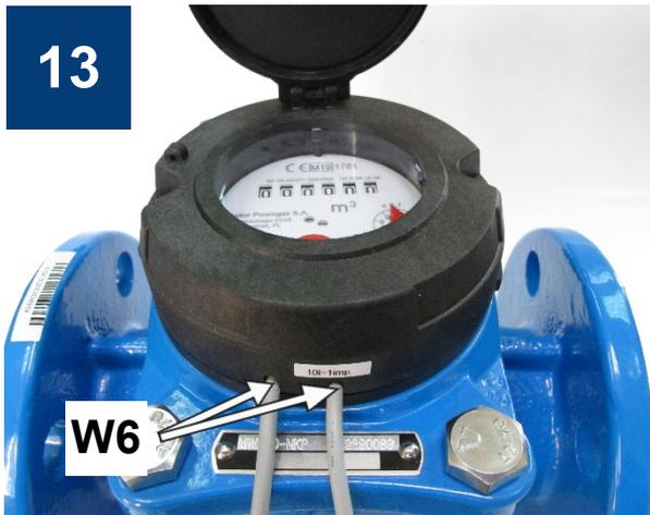
Install the counter guard assembly on the counter mechanism with the transmitter(s) installed so the transmitter cables go out of the counter guard via the respective cable entries (see view W6). The NK transmitter two-core cable should go under the “10 L = 1 pulse” label. Secure the counter guard with the two Allen bolts.
