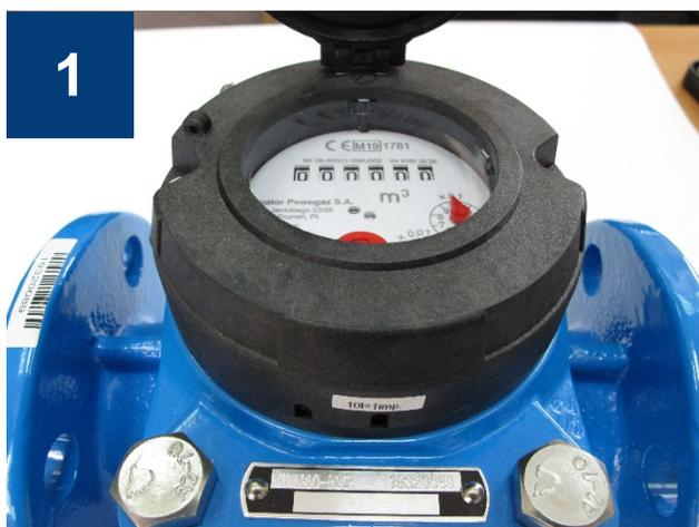
MWN40-NKOP water meter (NK and/or NO transmitter installation ready). The IP65-rated rotating counter features a single-magnet fixture installed at the x 0.001 position -> pulse rate at 10 L = 1 pulse.
