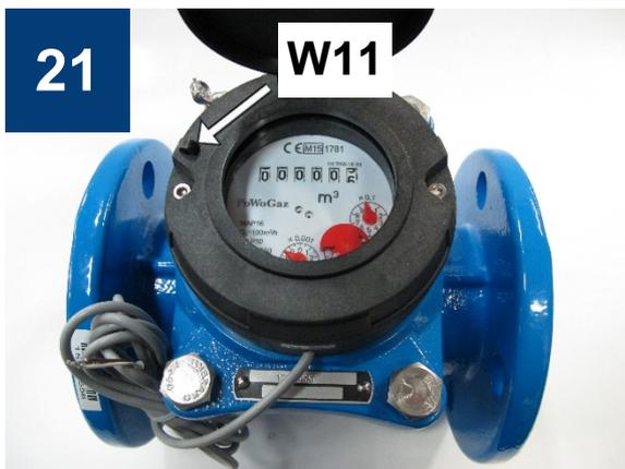
Install the counter guard assembly on the counter mechanism with the transmitter installed so the transmitter cable goes out of the counter guard via the respective cable entry at the “100 L = 1 pulse” label. Secure the counter guard with the two Allen bolts. Install the Allen bolt for the lead tamper seal wire in the hole next to the guard cover lug W7 in the counter guard to facilitate sealing of the water meter.
