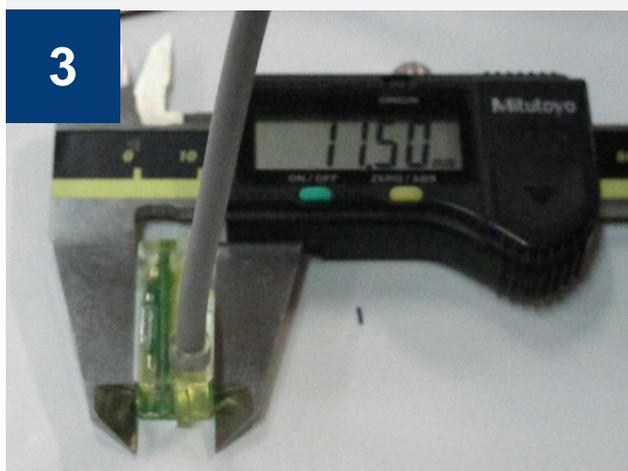
NK transmitters, P/N **31-8027-010000**, width  $b = 11.5$  mm for IP65-rated water meters. Specification:  $U < 30\text{VDC}$ ;  $I_s < (\text{max } 100 \text{ mA})$ ; cable: YTTY  $2 \times 0.14 \text{ mm}^2$ ,  $L = 2 \text{ m}$
